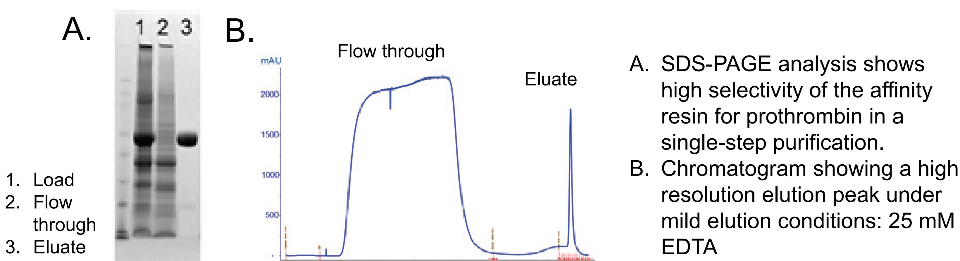
During the anion exchange chromatography process, the uncarboxylated variants of prothrombin elute in the pre-peak (AEC-HPLC). Comparison between anion exchange (QFF) and V<sub>H</sub>H affinity chromatography shows the V<sub>H</sub>H affinity resin has a very high selectivity for the most biologically active form of prothrombin. The single-step purification results in significant lower host cell protein content in the eluate, without compromising purity.
