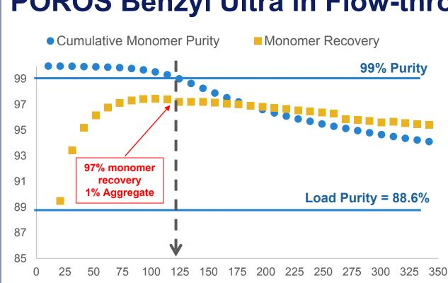
**Complete Aggregate clearance achieved with POROS Benzyl Ultra at low salt and flexible pH**
