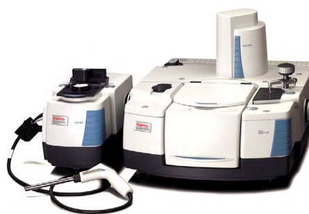
Thermo Scientific Nicolet iS50 FTIR Spectrometer, equipped with the iS50 NIR module
