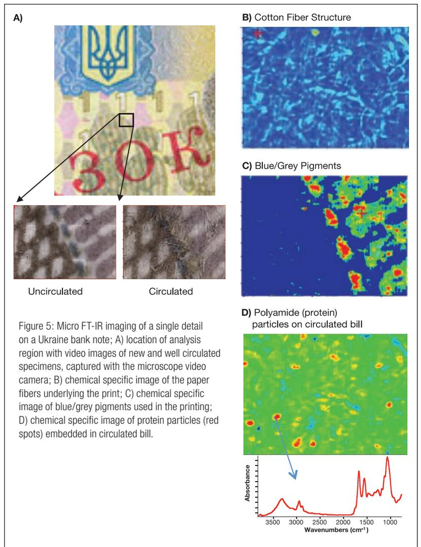
Figure 5: Micro FT-IR imaging of a single detail on a Ukraine bank note; A) location of analysis region with video images of new and well circulated specimens, captured with the microscope video camera; B) chemical specific image of the paper fibers underlying the print; C) chemical specific image of blue/gray pigments used in the printing; D) chemical specific image of protein particles (red spots) embedded in circulated bill.
