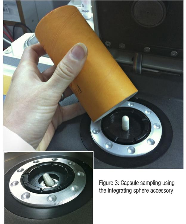
Figure 3: Capsule sampling using the integrating sphere accessory
