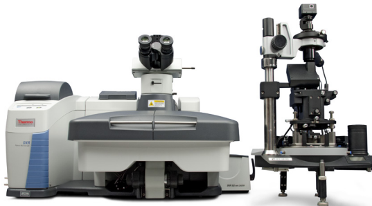
Figure 1: Thermo Scientific DXR Raman microscope integrated with an NT-MDT atomic force microscope
