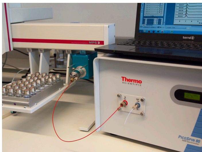
Figure 1: Low-field picoSpin 80 1 H NMR spectrometer with a MultiPurpose Sampler (GERSTEL) for automated sample preparation and injection of fuel samples for determining the research octane number (RON).
