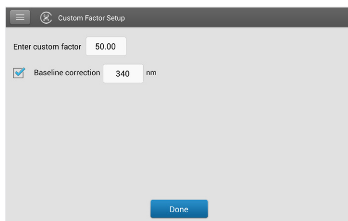
Figure 4. Custom Factor setup screen on the NanoDrop One/One c instrument (local control) software.
