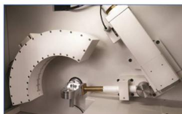
The ARL EQUINOX 100 and ARL EQUINOX 1000 provide very fast data collection times compared to other diffractometers due to their unique curved position sensitive detector (CPS) that measures all diffraction peaks simultaneously and in real time. Geological or mining samples for XRD measurements are typically powders which are ground to suitable particle size.
