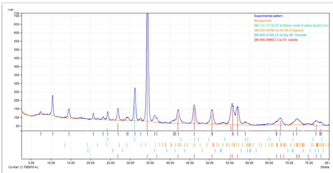
N.R.: The largest peaks with red vertical sticks are all Calcite = Limestone. Quartz peak is identified (blue vertical stick)
