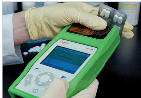
The TruScan GP analyzer can be used in the field to provide rapid identification of counterfeit pharmaceuticals.
