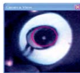
Figure 1: Eye feature on a painted object through the lens of the Niton analyzer CCD camera; 3 mm spot collimation allows you to isolate and analyze areas of interest.
