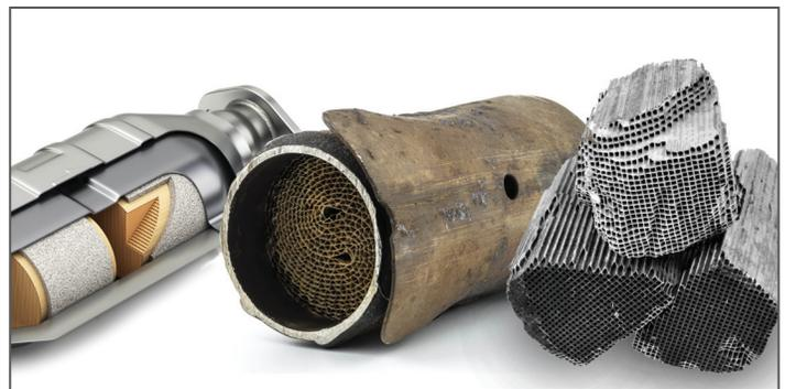
The physical recycling begins with decanning, or the removal of the shell and extraction of the honeycomb-shaped material inside the catalytic converter.
