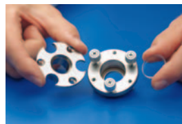
10 m cell window holder disassembled
