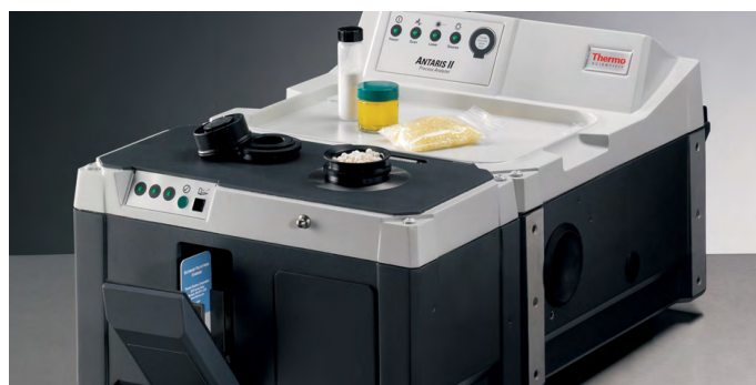
Figure 3: The Antaris FT-NIR Solid Sampling System is configured in this photograph to collect reflectance data through the bottom of a sample vial filled with lactose powder.
