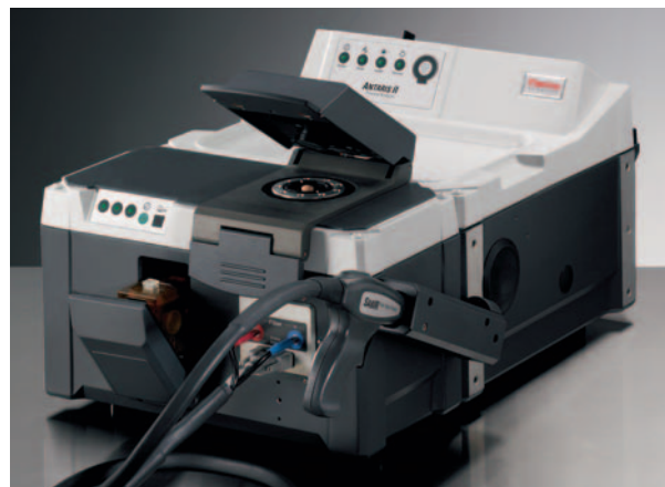
Figure 1: Antaris FT-NIR Method Development Sampling System
