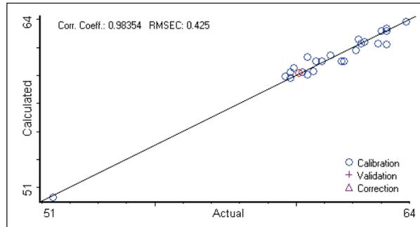
Figure 3: Calibration curve for choline chloride
