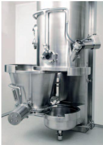
Figure 4: Fluid Bed Dryer
