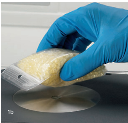
Figure 1. Antaris II MDS FT-NIR analyzer with integrating sphere (1a). The prepared samples were placed on top of the window over the integrating sphere, similar to what is shown in 1b, for the duration of the experiments.
