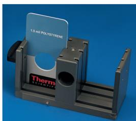
Figure 1: Three-position cardholder
