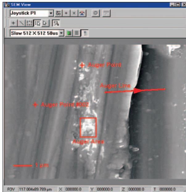
Figure 2: SEM image of part of a steel sample with analysis positions superimposed on the image
