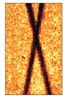
Figure 3: C 1s image of the PET substrate. Image collected in 5 minutes.
