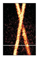
Figure 1: C 1s image of the carbon fiber. Image collected in 5 minutes.
