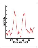
Figure 2: A line scan extracted from the C 1s image of the fiber, showing that the spatial resolution in the image is better than 2  $\mu$ m.
