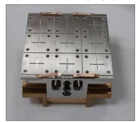
Figure 4: The sample holder for K-Alpha.
