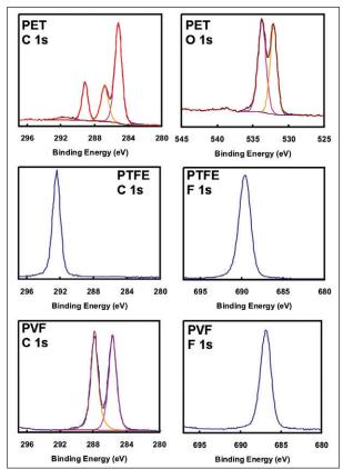
Figure 9: C 1s spectra from a series of polymer surfaces
