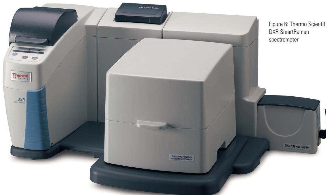
Figure 6: Thermo Scientific DXR SmartRaman spectrometer
