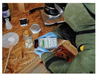
The FirstDefender RM unit can analyze through sealed containers without disturbing the sample.
