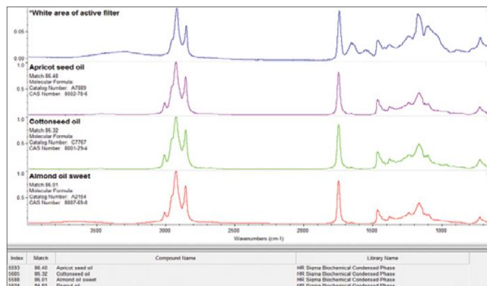
**Figure 4:** White material on the filter is a fatty acid (triglyceride).
