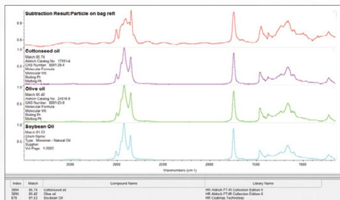
Figure 8: Subtraction results allowing identification of edible oil.
