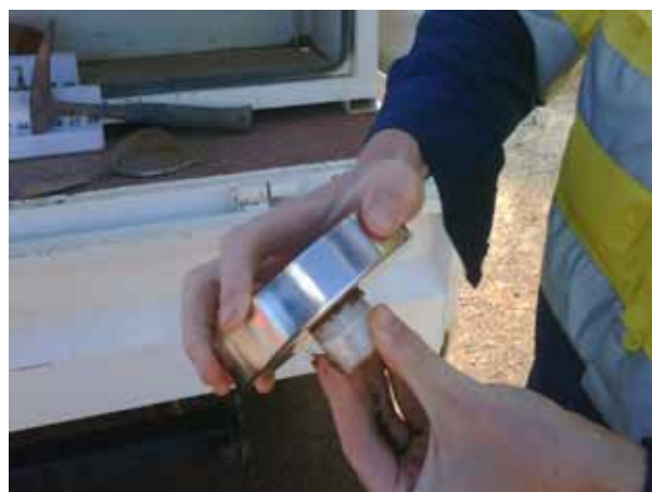
Figure 1. RC pulp sample is lightly pressed to make a flat surface for analysis.
