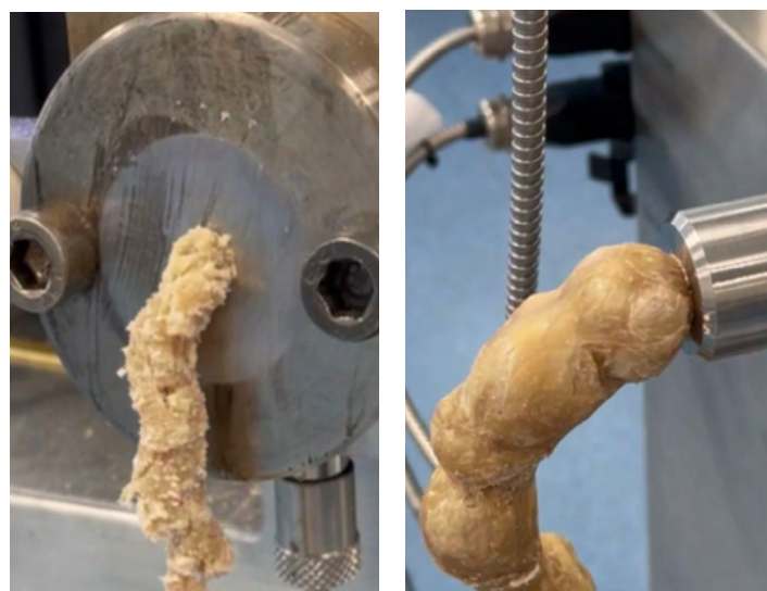
Figure 2. Soy protein concentrate with 33.3 wt% added water, extruded with a 16 mm length die (left) and a 40 mm length die (right).
