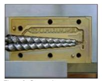
Figure 2: Co-rotating screws a) PE melt
