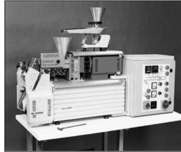
PRISM TSE 16 PC Powder Coating Extrusion line
