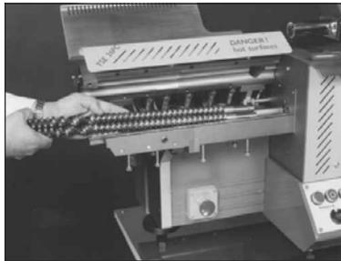
Screw removal from PRISM TSE 24 PC
