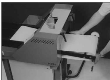
Removable Belt Cartridge on PRISM Chill Rolls
