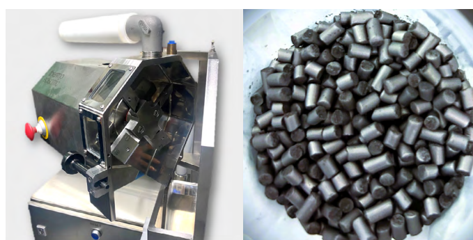
Figure 6: FaceCut 16 Pelletizer (left) cuts extruded paste into pellets (right) with rotating blades directly at the die exit.
