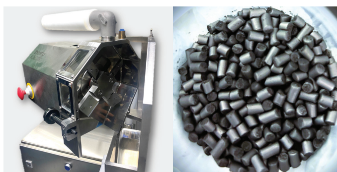
Figure 6: FaceCut 16 Pelletizer (left) cuts extruded paste into pellets (right) with rotating blades directly at the die exit.
