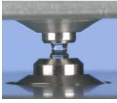
Figure 1a: Loading 1ul sample.
