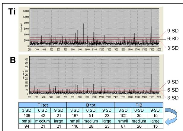
Calculating the inclusions between consecutive threshold values provides the number of inclusions in the size class that they delimit. In the example, the number of peaks and coincidences between 3 and 6-SD correspond to small size inclusions, between 6 and 9-SD to medium size inclusions and higher than 9 to large size inclusions. Such calculations allow generating qualitative inclusion size distributions.
