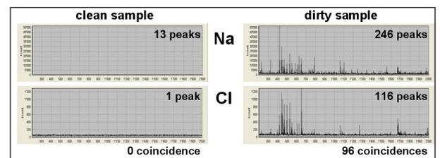
The algorithm *Composition* allows counting coincidental peaks, i.e. peaks appearing on the channels of several elements concurrently during the same single spark. The coincidence of a peak on Na and Cl channels means that these two elements are part of the same inclusion, for instance a sodium chloride (NaCl) inclusion. In the previous example, no NaCl coincidence was counted in the clean sample and 96 were counted in the dirty one.
