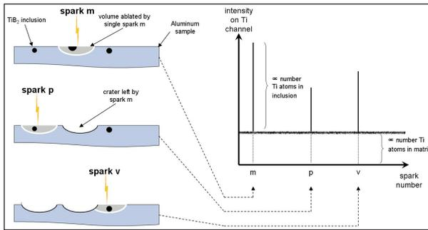
The intensity of the flat, noisy baseline signal is proportional to the concentration of Ti atoms dissolved in the matrix and the intensity of a peak depends on the amount of Ti atoms contained in the inclusion(s) ablated by a single spark. Consequently, the number of peaks is related to the number of such inclusions and their intensity to such factors as the inclusion size and the concentration of Ti in the inclusion.
