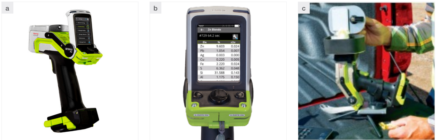
Figure 1. a) Niton XL5 Plus analyzer ; b) Display of results for elemental analysis of Zn-Pb-Cu-Ag ore; c) Sample analysis using the Thermo Scientific™ XL5 Mini Test Stand.
