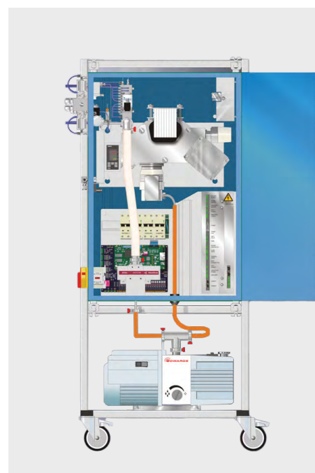
Figure 5: The Prima PRO Process Mass Spectrometer with the multipoint variable pressure inlet attached.
