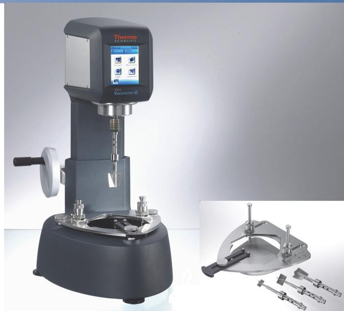
Fig. 1: Thermo Scientific HAAKE Viscotester iQ with mounted universal container holder and vane rotor FL26-2 blades (left); universal container holder with three vane rotors: 4-blade rotors FL16 and FL22 as well as FL26-2 blades (right)
