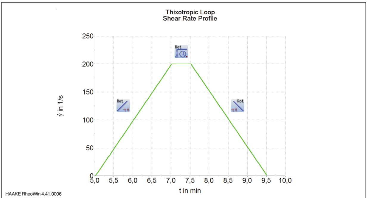
Fig. 3: Shear rate profile for the so-called "thixotropy loop" consisting of an up ramp, a peak hold time at the maximum shear rate and a down ramp.
