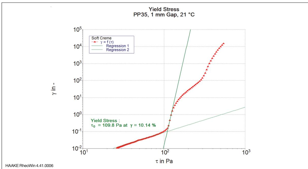
Fig. 5: Deformation as a function of stress for the soft cream sample. The yield stress is calculated as the point of interception of the two green tangents, marking the transition from elastic deformation to viscous flow.
