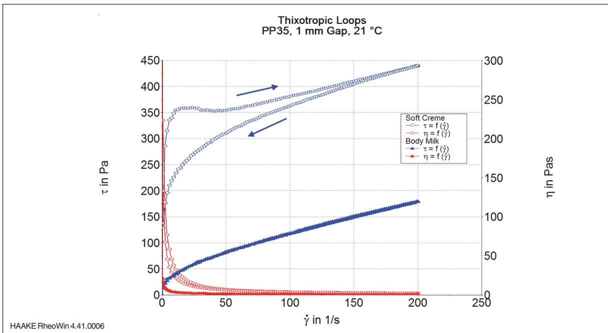
Fig. 4: Results of the thixotropy test for soft cream (open symbols) and body lotion (filled symbols). The soft cream shows a thixotropic behaviour, indicated by the clear difference between the up and down part of the flow curve. The up and down curve for the body lotion are identical, thus the sample is not thixotropic.
