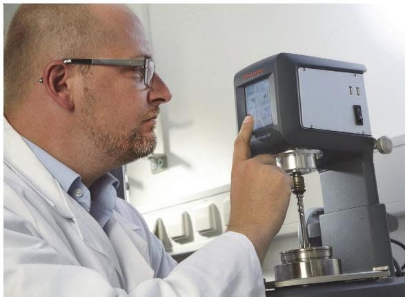
Fig. 2: HAAKE Viscotester iQ used as a standalone unit with internal measuring procedures, HAAKE Viscotester iQ RheoApp for extended measuring capabilities
