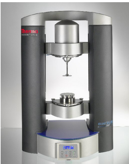
Figure 1: The HAAKE MARSTM Rheometer.
