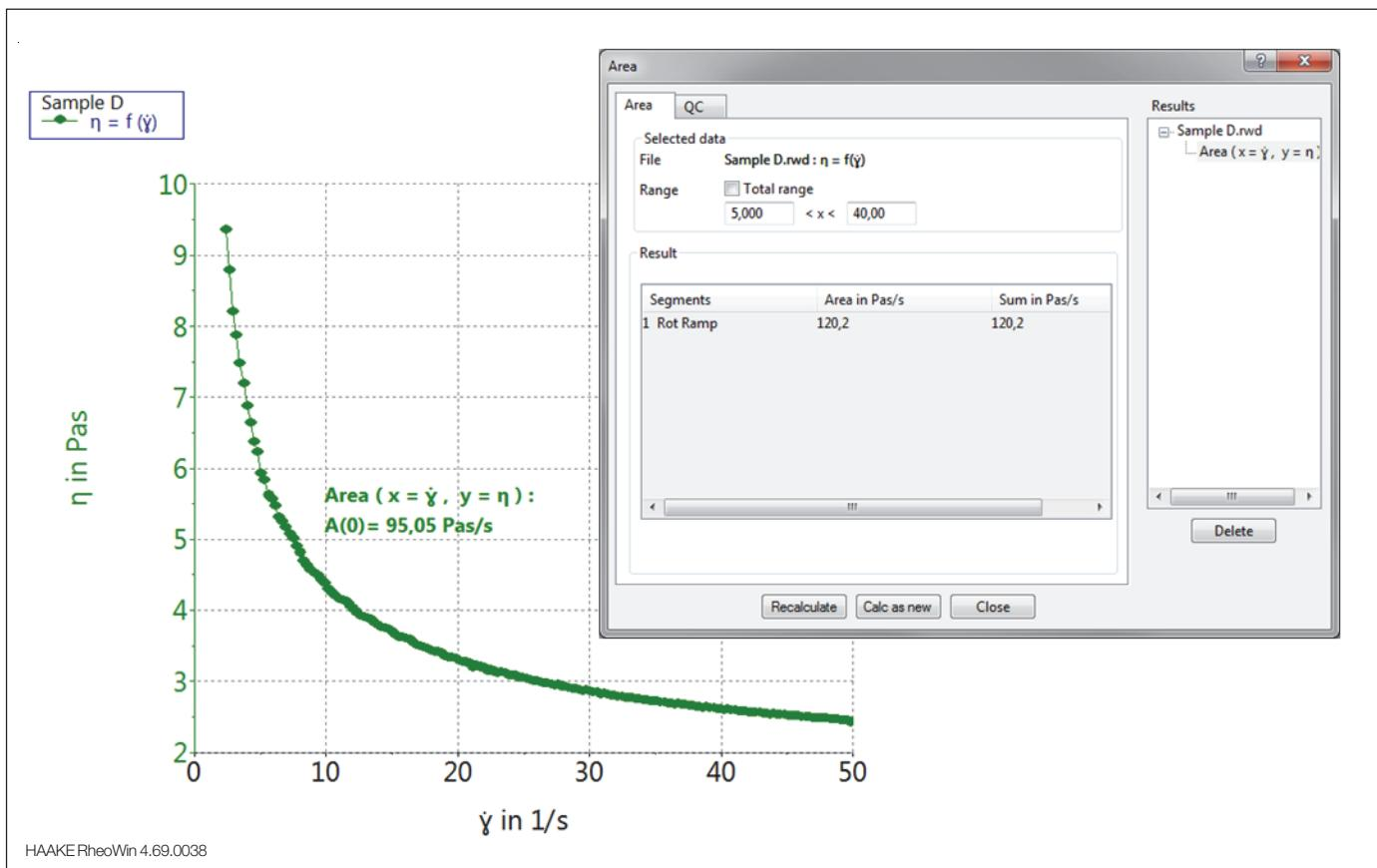
Fig. 7: Calculating the area under a viscosity curve.
