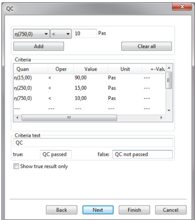
**Fig. 2:** Definition of Quality Control criteria in a measurement and evaluation routine.
