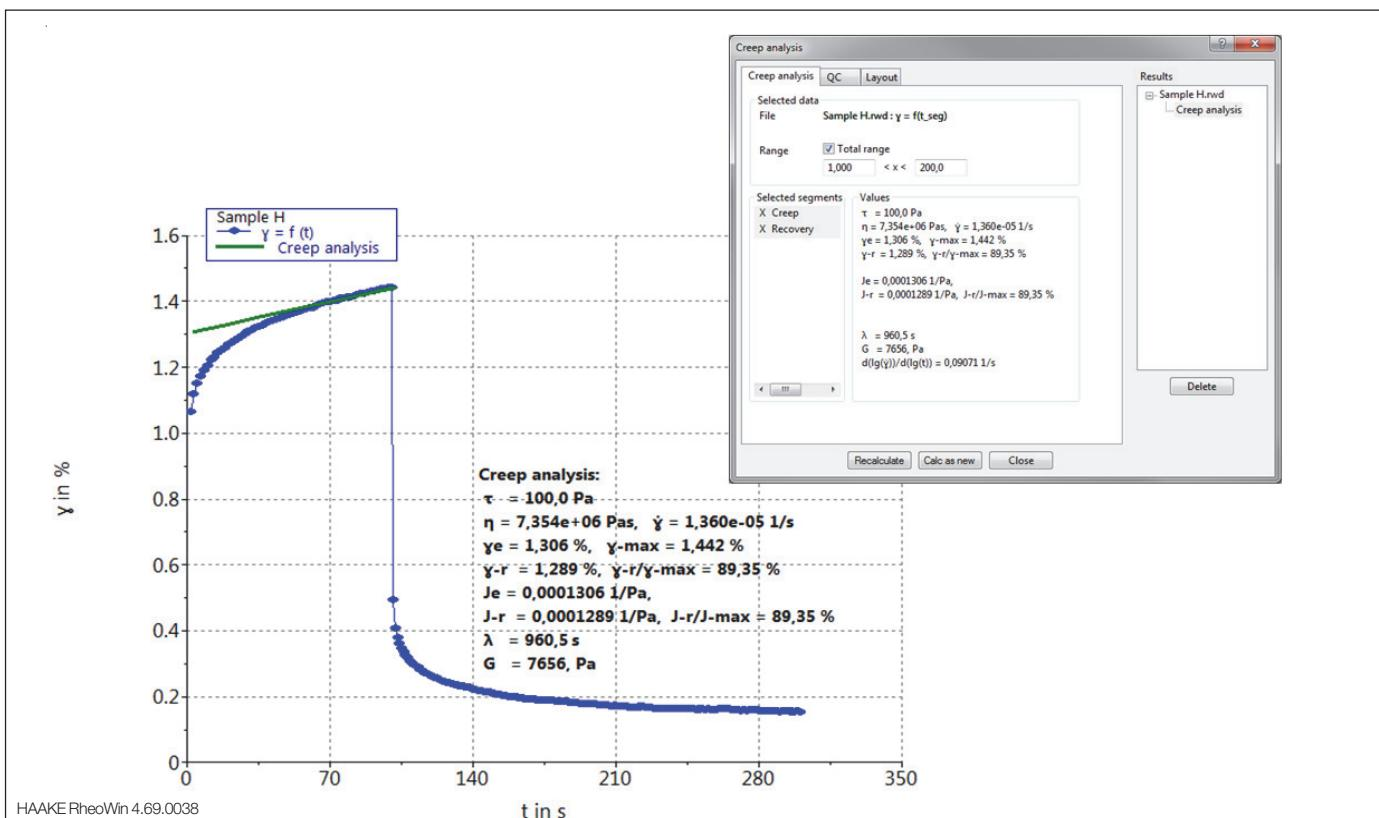
Fig. 14: Analysis of a creep and recovery test.
