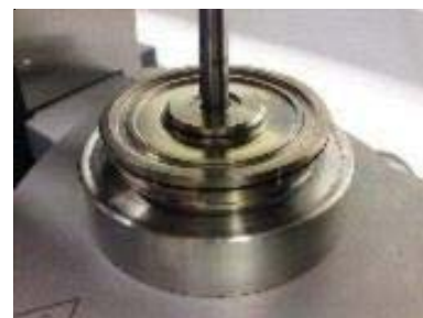
Fig. 7: Lower measuring plate TMP with a diameter chosen to match the upper geometry
