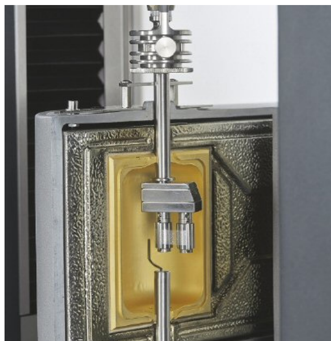
Figure 1: Controlled Temperature Chamber (CTC) of the HAAKE MARS Rheometer with the SER tool.
