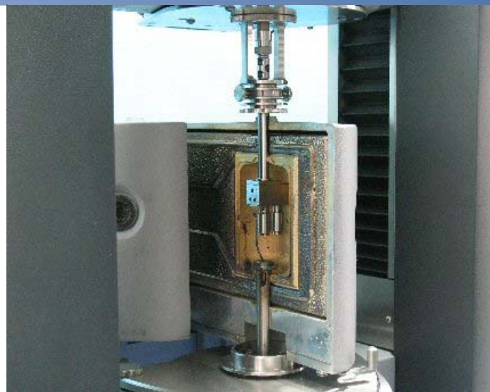
Fig. 1: Controlled Temperature Chamber (CTC) of the HAAKE MARS with the SER.
