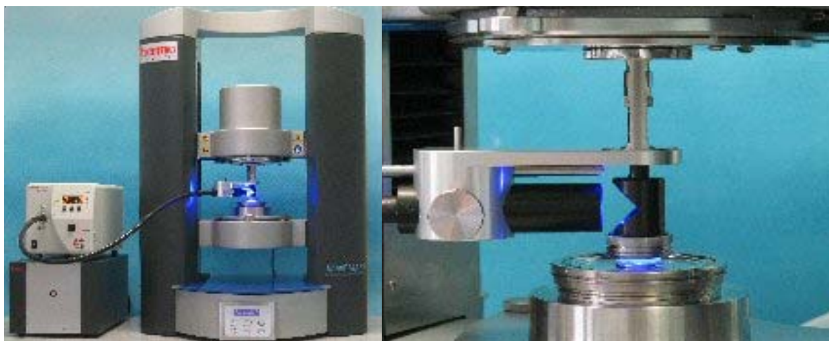
Fig. 3: The HAAKE MARS III equipped with the Upper Plate UV Tool (left). The sample is exposed to the UV light from the top through a UV transparent rotor (right). For these photos the sample hood usually used for safety reasons and better temperature control has been removed.
