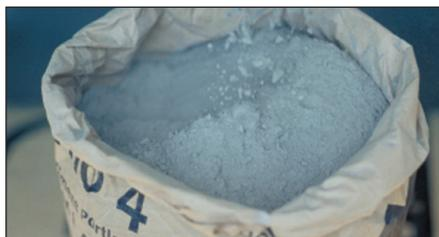
For use in Portland cement, fly ash must meet the requirements of ASTM C618, which separates the material into two classes (F and C). These classes differ in the amount of calcium (Ca), silica (Si), aluminum (Al) and iron (Fe) content.
