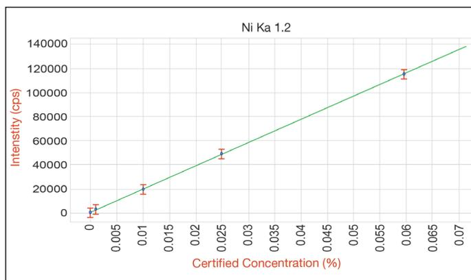
Figure 2: Calibration for nickel in diesel fuel oil SEE = 0.025 ppm
