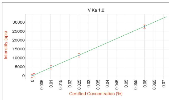
Figure 1: Calibration for vanadium in diesel fuel oil SEE = 0.020 ppm
