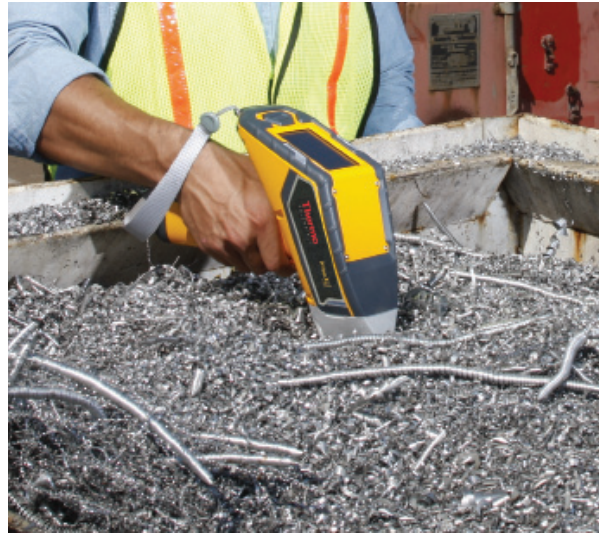
Thermo Scientific Niton XL2 GOLDD and Niton XL3t GOLDD+ analyzers deliver rapid analysis and grade ID
