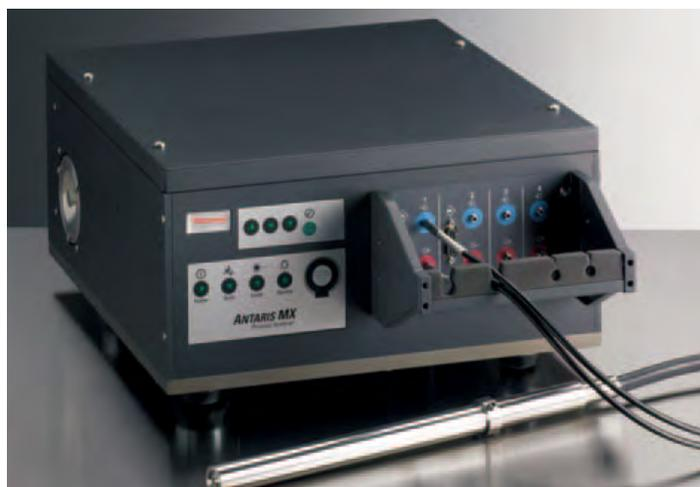
**Figure 1: Antaris MX FT-NIR Analyzer used for the collection of media dissolution spectra**
