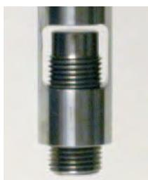
**Figure 2:** Transreflectance probe used in the analysis, showing detail of adjustable pathlength.
