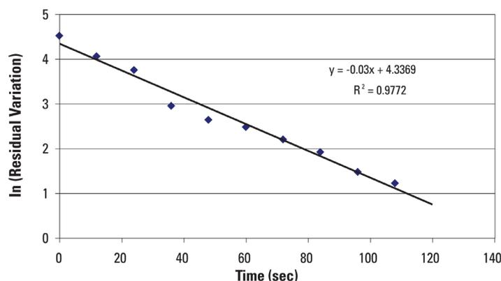
Figure 6: Kinetics plot showing the dissolution of the media follows a first-order rate law. Dissolution half life ( $t_{1/2}$ ) is calculated as approximately 23 seconds.
