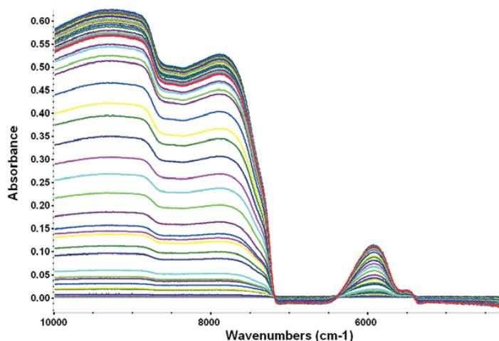
Figure 4: Spectra tracking dissolution of media over time. Spectra were ratioed against a water background.
