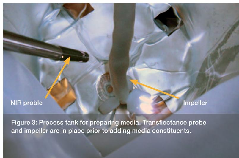
**Figure 3:** Process tank for preparing media. Transreflectance probe and impeller are in place prior to adding media constituents.
