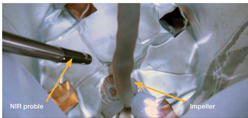
Figure 3: Process tank for preparing media. Transreflectance probe and impeller are in place prior to adding media constituents.
