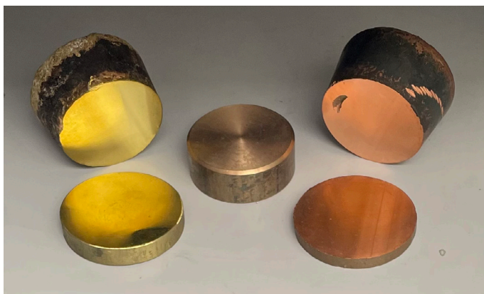
Figure 2: Brass, bronze and copper samples.
