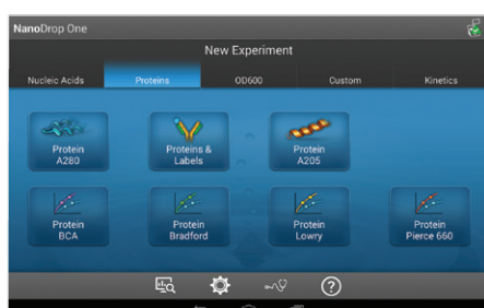
Figure 1. NanoDrop One Proteins Home screen showing available preprogrammed applications for protein quantitation.
