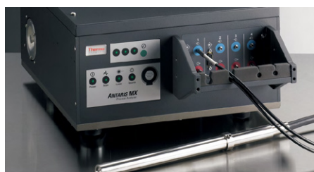
Figure 1. Antaris MX FT-NIR Process Analyzer used for collecting the spectroscopic information from the cell cultures.
