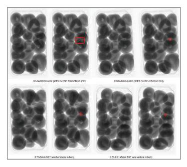
Testing proved smaller sizes of standard metal spheres, needles and wires were detected by the X-ray system. All metals were tested in many orientations (vertically, horizontally in direction of flow, horizontally perpendicular to flow and at angles) to ensure successful
